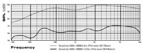
The RCS5FT/EN & ENC have been tested for 100 hours at a maximum power of 6W. Both units did not deviate by more than +/- 3dB. The frequency response and impedance curves remained constant throughout the test period. All results are in full compliance with the requirements of EN54-24.
