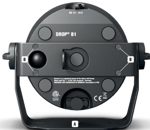
In order to effectively use the tilt function with the tilt screw when using as an upright, and to achieve a more inconspicuous look, you must use a suitable tool to remove the mounting bracket by releasing the four T10 Torx screws (B) that secure the mounting bracket to the spotlight housing.
