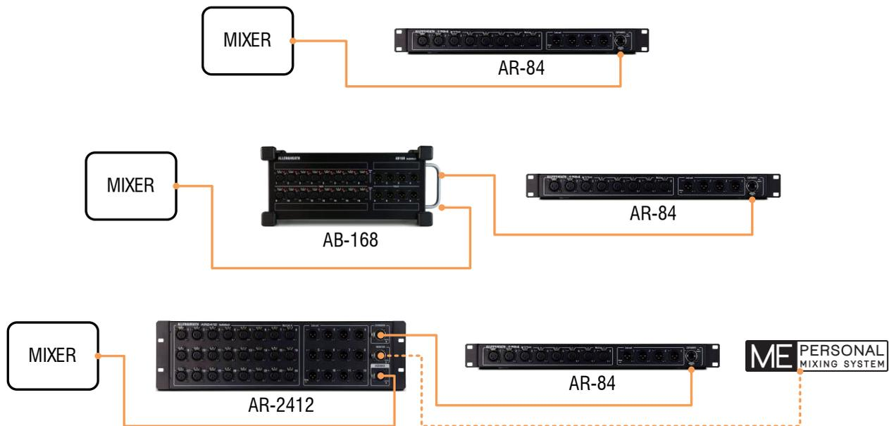
ⓘ A maximum of two dSnake remote units can be connected to each mixer's dSnake port.
