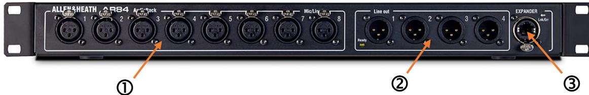
① **Input sockets** 8 balanced XLR mic/line inputs. The preamps are built into the **AR84** and their Gain, Pad and 48V phantom power are controlled remotely from the mixer via the dSNAKE link. Refer to mixer documentation for information on patching these sockets to input channels or other destinations in the system.
