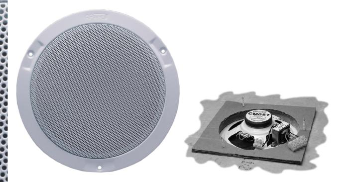
The APart CM6ST is a metal ceiling loudspeaker. The treated dual cone 6.5" loudspeaker is very suitable for all evacuation and paging purposes. The loudspeakers is equipped with a high quality 6 watt 100 Volt transformer with different power tappings.
