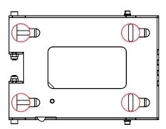
**2** Loosen the four hexagon socket screws from the subwoofer (see markings). Attach the four enclosed rubber pads to the subwoofer using the loosened screws.
