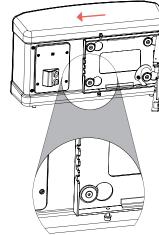
4 Step 1: Loosen the two locking screws (unscrew approximately 7 mm from the thread; do not remove). Step 2: Open the mounting bracket and place the safety hook over the rubber pad (push the lever towards the arrow as far as possible) to prevent the subwoofer from accidentally slipping out of the bracket.
