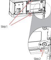
**5** Carry out the cabling (description in the user manual for the corresponding subwoofer) and push the cables into the appropriate cable cut-outs. Close the mounting bracket (fold the subwoofer) and tighten both locking screws. The safety hook cannot be released when the mounting bracket is closed.
