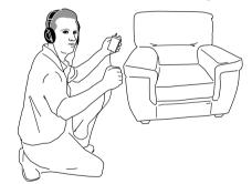
When you are satisfied with the signal in the centre of the loop, move around the room to ensure coverage is consistent throughout. Pay particular attention to areas where the hearing aid user is likely to sit. Next, if possible with the hearing aid user in position, set the amplifier's tone and microphone controls to suit their personal preference following steps 6 and 7.
