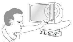
Turn on the system's audio input source (usually a television and/or a microphone) and ensure it is producing an audio signal. Note, SCART outputs have a fixed level signal and altering the TV's volume control will not affect this.
