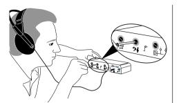
6 Adjust the tone control to suit the user. Turning the control clockwise usually improves speech intelligibility and makes the sound more 'natural'. Turning it anticlockwise makes the sound 'warmer'. Large turns in either direction may lead to you having to adjust the loop signal control accordingly (see step 4).
