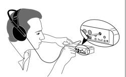
If two microphones are used, more emphasis can be given to one over the other by turning the amplifier's microphone priority control clockwise or anti-clockwise to suit. When the control is in the centre position (its default setting), equal emphasis is given to both microphones.
