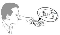
Check that the loop strength meter is not permanently lit red. The meter is designed to light progressively from 1 to 3 (green to yellow to red) in line with the loop signal strength. If it is continually lit red, the signal will be distorted and the amplifier may overheat. If necessary, re-adjust the loop signal control accordingly and re-test the sound quality following steps 4 and 5.
