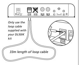
Connect the loop cable by pushing one of its prepared ends into the left terminal and the other into the right terminal. The push-and-hold connectors will automatically grip the ends. Any excess cable should be neatly tied up and placed where it cannot be tripped over. If you need to remove the cable at any time, you must first insert a terminal screwdriver into the rectangular hole directly below the cable insertion hole (see right). This will
