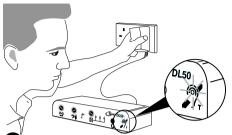
With all system connections in place (see pages 6 & 7), apply power to the amplifier and check its green 'power on' indicator is lit.
