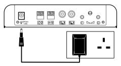
Only use the plug-top power supply supplied with your DL50 kit. Note that there are no user-servicable parts on this power supply and in the event of failure you must purchase a replacement lead. Refer to the ancillary order form attached for details.
