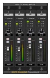
The window shows the controls and indicators for the 4 analogue inputs that the unit can receive using its rear panel balanced terminals, and that will be converted to 4 Dante Channels:
