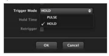
• **PULSE**: the priority audio will start playing in the destination players (A / B) when the trigger stimulus appears and will keep playing for the time defined by the Hold Time parameter. When Retrigger option is enabled, a new trigger pulse happening during the Hold Time period will start the event again from zero, resetting the time counter as well.
