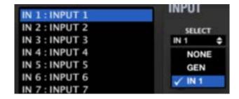
That means: INPUT 1 in the matrix processing can just take its signal from the internal generator or the audio source physically connected to IN1 back panel terminals. The same happens with INPUT 2  $\rightarrow$  IN2, INPUT 3  $\rightarrow$  IN3, ..... INPUT 9  $\rightarrow$  DIN1, INPUT 10  $\rightarrow$  DIN2, etc. (Digital inputs can be Dante or AES67)
