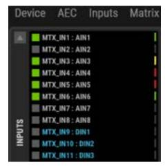
• **Green**: the input level has exceeded the noise gate threshold (opened gate) and the input is currently included in the automatic mix. Inputs 1 and 6 in this example.
