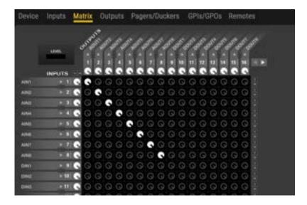
On the left side column, it shows the total of 64 audio INPUTS channels available in the matrix. The names of the inputs are the same defined as MTX\_Inn: **custom label** in the INPUT section.
