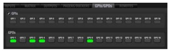
MIMO88's GPI and GPO ports allow you to connect external control hardware and to interact with these units: potentiometers, push buttons, limit switches, lights, motors, etc.
