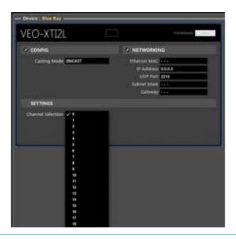
Each VEO-XTI2L transmitter must be settled with a unique channel number in the same network. If two transmitters are transmitting on the same channel, they will create network conflicts.
