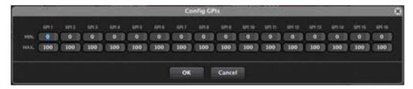
Example for calibrating a WPmVOL / WPaVOL hardware potentiometer connected to GPI #2 to remotely manage a volume control of MIMO88:
