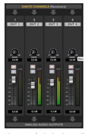
It shows the controls and parameters for the 4 analogue audio outputs that the unit delivers at its 4 rear panel balanced audio output terminals, which take their contents from the 4 Dante channels received in the unit from the network, through the RJ45 connector:
