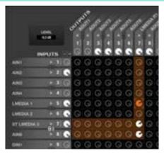
In the above example we can manage 3 media audio sources for our Local Media contents in Room 1. Note that the ST to mono conversion is as well managed automatically.
