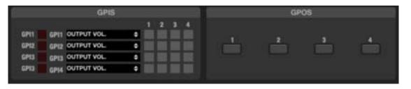
The unit's **GPI** ports (0-10 VDC control ports) on the rear panel are displayed as GPI 1 to 4. To the right of each of them is displayed the value of the signal (voltage) received on the central pin of each GPI port, read in real time (0 to 100 scale). A WPm / WPa VOL or WPmVOL-SR / WPm / WPaVOL-SR wall panel, or similar, connected to a GPI will deliver this full range, 0 to 100 values, when gestured.
