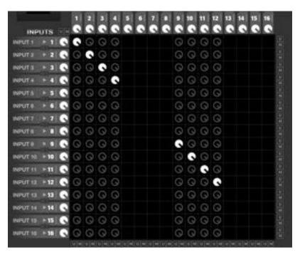
In this case it is possible to process up to 8 independent mixes (outputs 1 to 4 and 9 to 12) using any combination of the 16 available inputs as sound sources.
