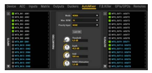
The AUTOMIXER processing module uses a very sophisticated algorithm to manage what input signals must be part of the automatic mix and under what conditions, and what signals must remain apart. The AUTOMIXER analyses the audio content on all inputs to identify what should be considered as background noise and what should be considered as a valid signal to trigger the input channel in the auto mix.
