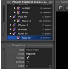
To add a control in a page, click with the right mouse button and select the type of control to add from the drop-down list:
