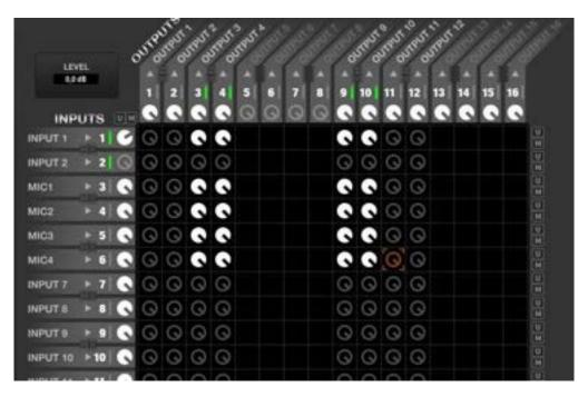
The picture above shows how inputs 1, 3, 4, 5 and 6 are routed toward outputs 3, 4, 9 and 10. Thus it would be possible that any selection of these inputs and outputs in the AUTOMIXER module could result in an automatic mixture according to the settings made in this module.
