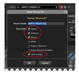
After a preset has been saved, with a given configuration saved in it, recovering the preset in the future means overwriting the current MIMO7272DN configuration with the "Save Data" options that were included in the preset at the time it was saved.
