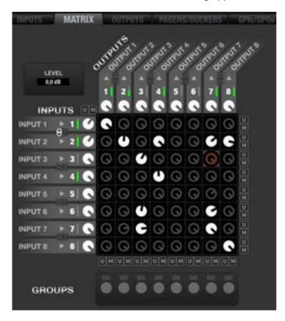
The matrix inputs are represented in INPUTS column, on the left, while the outputs are arranged in OUTPUTS row, at the top.
