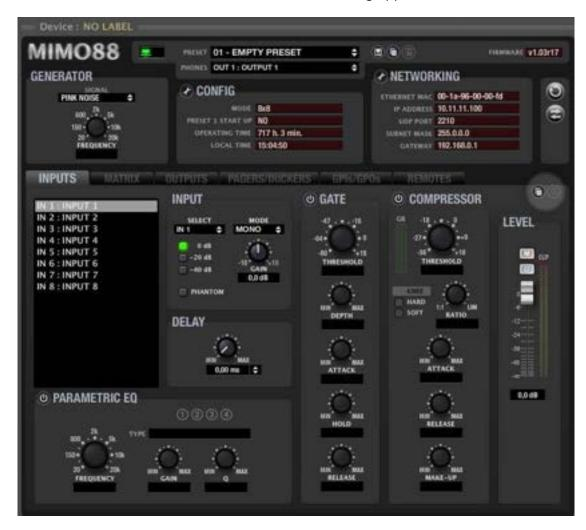
There are two distinct parts. A top section intended for unit general configuration and settings, and a series of tabs at the bottom (INPUTS, MATRIX, OUTPUTS, etc.) to show the different sections of the device programming.
