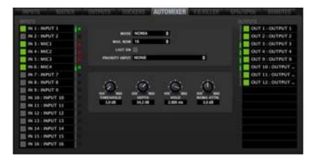
The AUTOMIXER processing module uses a very sophisticated algorithm to manage what input signals must be part of the automatic mix and under what conditions, and what signals must remain apart. The AUTOMIXER analyses the audio content on all inputs to identify what should be considered as background noise and what should be considered as a valid signal to trigger the input channel in the auto mix.
