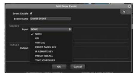
• **GPI**: a GPI can be activated by closing a contact between terminals +10VDC and n, where n can be GPI 1, 2, 3 or 4 (example activating GPI 3)
