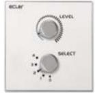
This type of control is connected to the MIMO88 unit via its GPI ports, not via the digital bus. A GPI port is required for the volume control and another one for the source selector. Additionally, you can connect an external switch (not included in the WPmVOL-SR / WPaVOL-SR) to a third GPI to perform the X-FOCUS MUTE function (muting the selected sound source).
