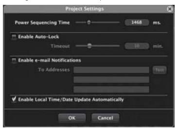
Power Sequencing Time (0 to 5000 milliseconds): sets the power sequence time delay between a device and following devices involved in the Project.
