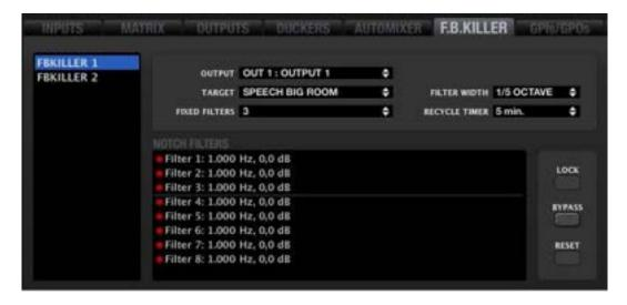
The FEEDBACK KILLER section consists of 2 banks, with 8 automatic filters in each one of them. The 2 banks are independent in terms of settings, operating mode and assigned output.
