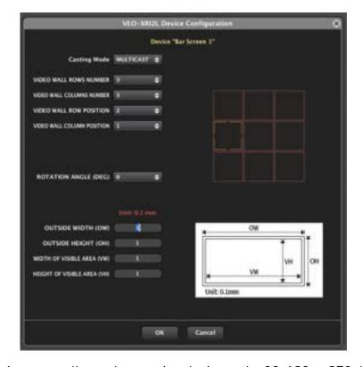
The configuration menu allows also rotating the image by 90, 180 or 270 degrees.
