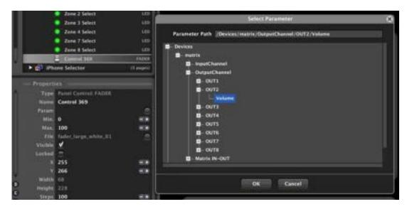
Then a browser window (Select Parameter) opens to select a hardware unit of the project and, within it, a parameter to control. Continuing the example above, the fader that is now displayed with its new appearance (large, white) will control OUT2 volume in a device called "matrix" (in this case a MIMO88).
