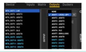
Whenever two or more Matrix Output Channels are routed to the same Output Port, this Output Port will get a direct mix of the Matrix Output Channels involved.
