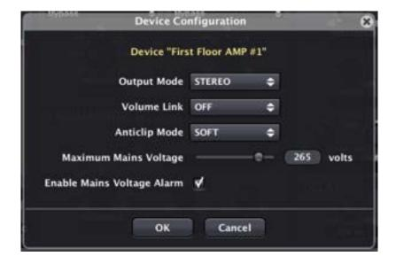
For an NPA Series amplifier, adjustable parameters are:
