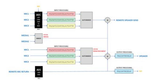
In each AEC ROOM CONFIGURATION window, it's also possible to select up to 2 LOCAL MEDIA: this allows sending non-microphonic local media contents (e.g. audio from a PC presentation or from an external AV player, but not audio from microphones in the room) to the REMOTE LOUDSPEAKER SEND (far-end) and to the LOCAL LOUDSPEAKER.
