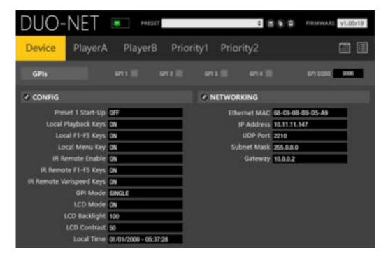
The GPI LEDs show the activity of the active / inactive GPI contacts at the back side of the unit. In the following image GPI #1 and #3 are ON (ON = connected to the "+" terminal by means of an external contact closure, or to an external voltage source, +10VDC).
