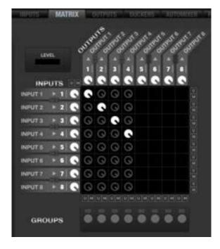
The image shows that the MIMO88CONF has the ability to process any mix of inputs you may have sent to one of the first 4 outputs on the unit. In other words, it is possible to generate up to 4 independent mixes, using any combination of the 8 available inputs as sound sources.
