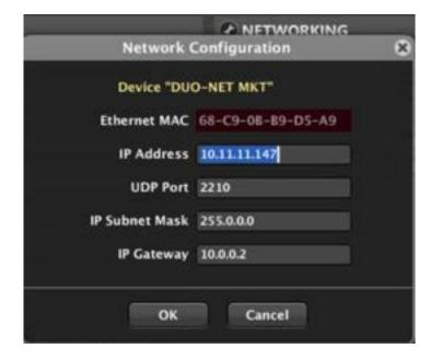
As every EclerNet device and computer belonging to an EclerNet project, the DUO-NET needs to get a manually configured static IP address and subnet mask.
