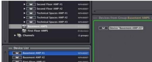
A device group provides both management and supervision (from the group control interface) of some controls concerning all devices in the same group (e.g. to sequentially turn on/off all group amplifiers by pressing the group *POWER* key).
