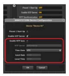
When NTP service is disabled or not available, the unit will keep the internal RTC (real Time Clock) running, without being able to automatically synchronize with an external reference clock service.
