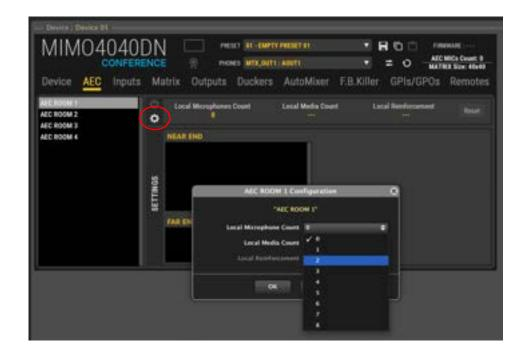
The AEC modules include a different and isolated processing and routing if compared with normal or "standard" input and output ports from the audio matrix. INPUT PORTS and OUTPUT PORTS selected in the AEC modules are not routed to the standard MATRIX (MATRIX section tab) in the MIMO unit. Matrix and AEC modules are independent and can work autonomously and simultaneously with different input / output signals.
