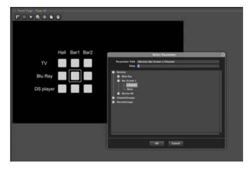
Each column represents a VEO-XRI2L receiver and each row represents a source identified by its related VEO-XTI2L transmission channel.
