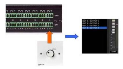
The picture is a representation of a WPVOL physically connected to the GPI 1 and assigned to the volume of MIMO88's output 8 by EclerNet Manager programming
