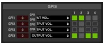
When a LEVEL control (software fader) and a GPI are associated to control the volume of the same input or output, both are concatenated ("in series"), so that the highest level of one of them at a given time will determine the maximum volume control that can reach the other when set to its maximum position.
