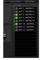
The inputs assigned to automatic mixing in the AUTOMIXER module must first be properly assigned in the MATRIX section, by adjusting the MUTE and level controls of its crossing points to correctly route them toward the desired outputs.
