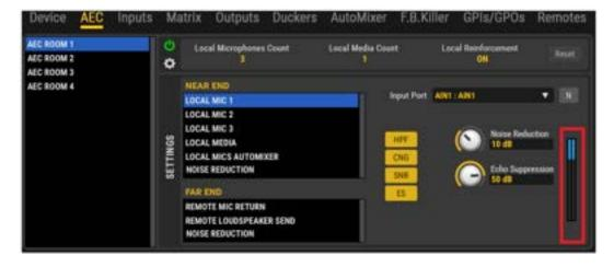
An optimal position of ERL is between the starting position and half scale. In case of full scale or negative values, it indicates issues on the gain structure.
