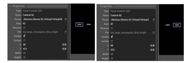
Please note that when a LED is linked to a parameter that can only take two values, 0 or 100, off or on, the Data field is unavailable because it's not possible to freely assign a specific value to light the LED. In the following example this happens when you link a LED to a MUTE function, which can only have two possible values:
