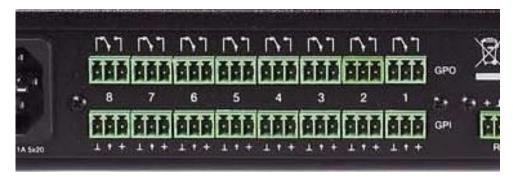
A GPI port (General Purpose Input) is a MIMO88 physical connection that lets read the DC voltage applied to it, and that can vary within the range of 0 to 10 VDC (0 to 100% in the
