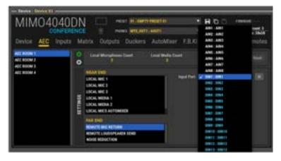
The input can be one of the 8 MIMO4040CDN analogue inputs or one of the 32 Dante™ / AES67 input channels. In order to make the project clearer, the label can be customized using the "N" button, like explained in the INPUT section of MIMO7272DN..
