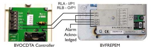
Note: The BVFREPEM includes a Normally Closed Fault Input between I/P 2 and O/P 2. These points must be linked to prevent a fault being announced.
