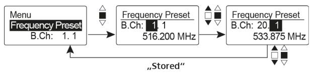
While you work in the **Frequency Preset** menu, the RF signal is deactivated.
