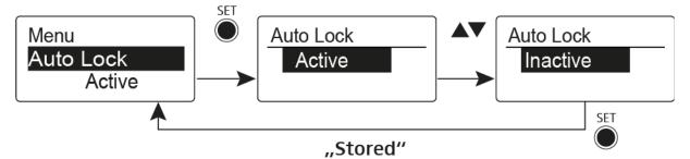
This lock prevents the bodypack transmitter from being unintentionally switched off and also prevents any unintentional changes to the transmitter's configuration. In the current standard display, the lock icon shows whether the lock-off function is currently switched on.
